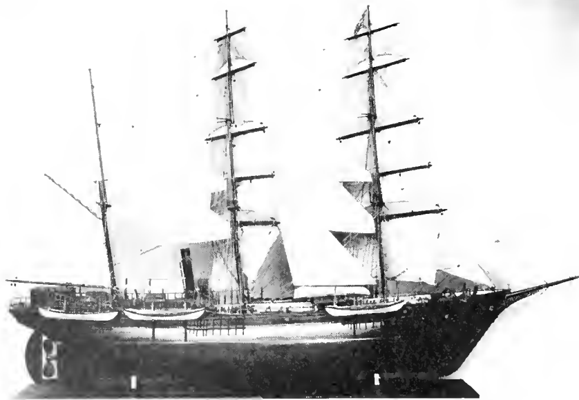
WHALING STEAMER Orca , built at San Francisco, California, in 1882. The largest of her type when built, and most completely fitted, her register dimensions were 177' x 32'6" x 18'11", 462.39 net tons, 280 horsepower. Abandoned off Point Barrow, Alaska in 1889. Rigger model USNM 76237. (Smithsonian photo 26758 h.)
